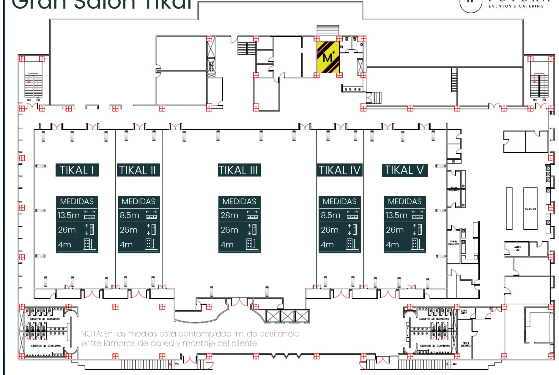
**M\*** Monta cargas: 5.0x3.6x2.5m / 10TON
